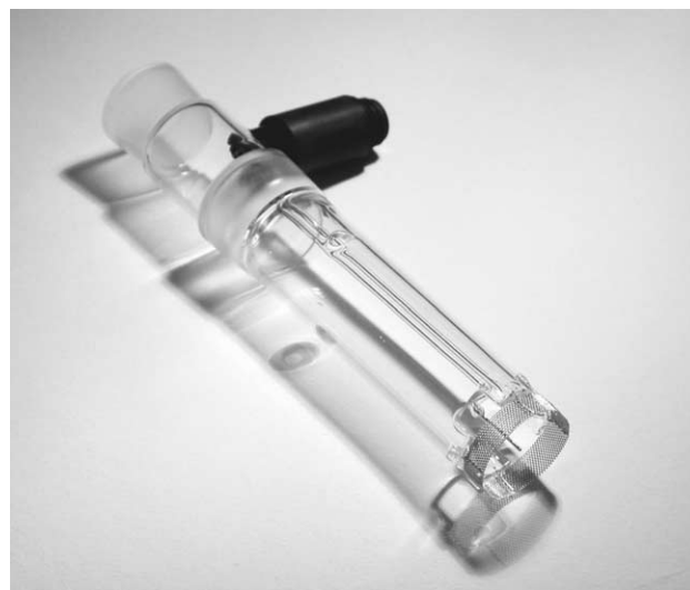
Fig. 2. Diaphragm-free current generator for the METTLER TOLEDO DL32/DL39 coulometer.
